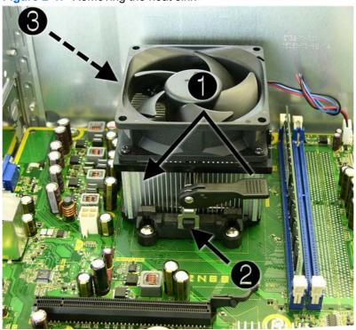
Figure 2-47 Removing the heat sink
